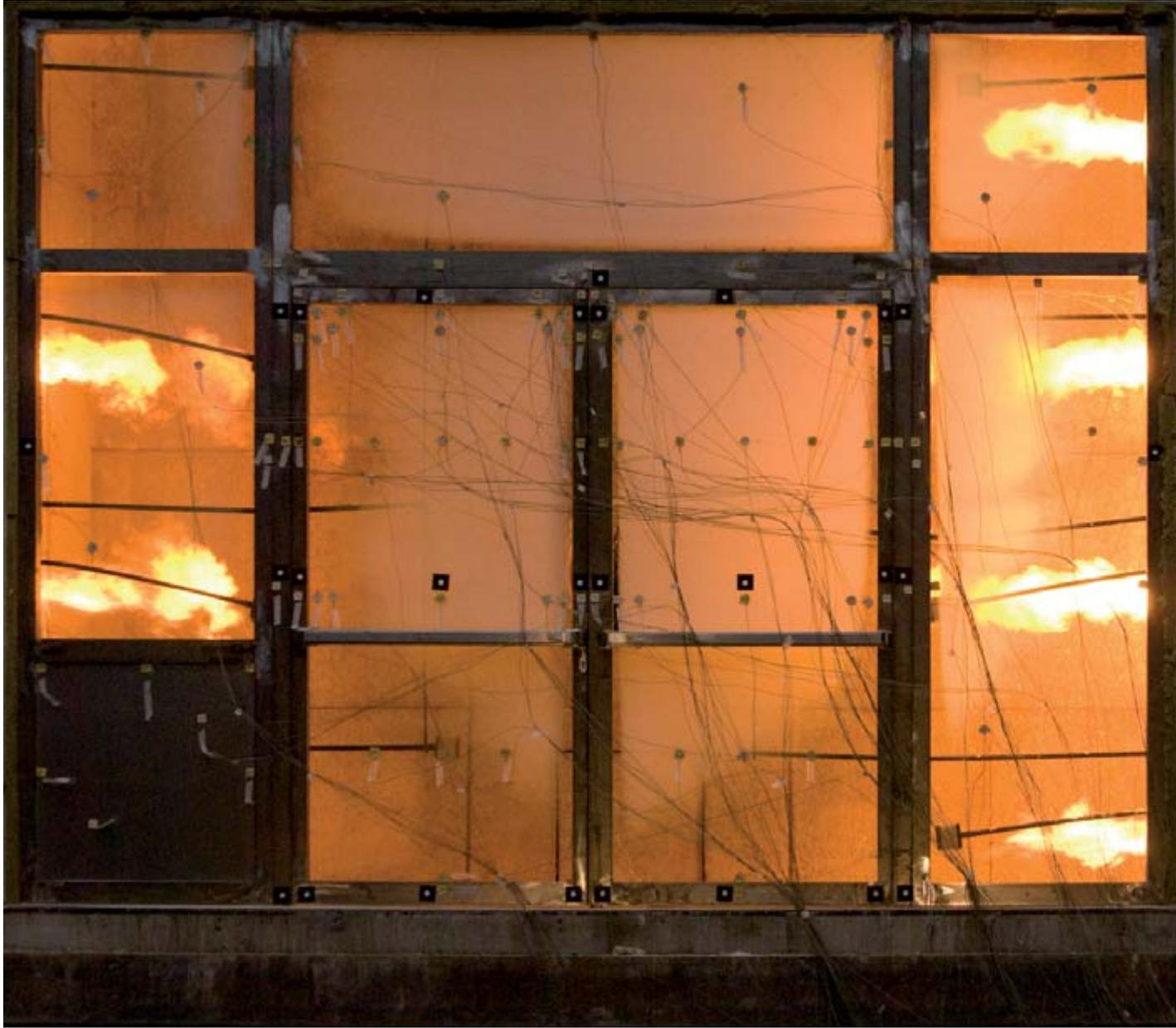
The ability of a door or a window frame to resist to the high stress induced by a fire is tested in specific labs equipped with special burners and tools following strict European procedures. The test is performed on a real-size specimen in which all components - profiles, glass, seals, locks, door closers - are tested in real conditions of use after being
