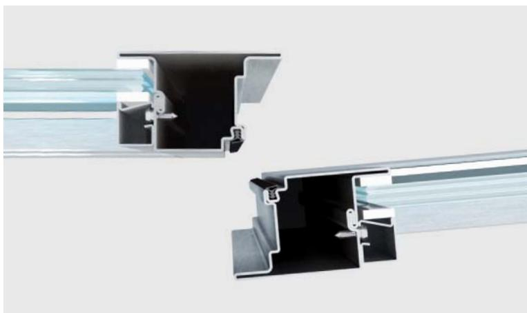
The ability of not letting fire or hot fumes through (fire resistance E) is guaranteed by the particular structure of the profile and by a rebate double seal system. The ability to keep the irradiation from the side not exposed to the fire (irradiation W) is guaranteed by special glass provided. The performance of AF Ew 30/60/90 system has been tested by the best European certifying labs under the reference standards EN 1634-1.
