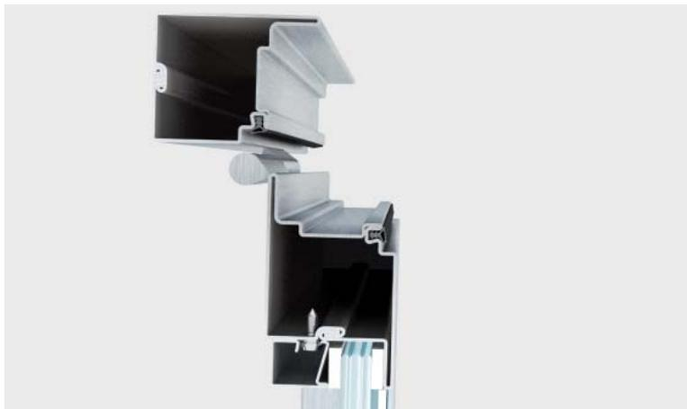
AF Ew 30/60/90 is an integrated system with accessories, seals and thermally non-insulated profiles 55 mm deep allowing for a wide range of fireproof doors and glazed partitions. They can be equipped with single or double glazing up to 35 mm thick. Each solution is equipped with a related set of certified accessories integrated in the system.
